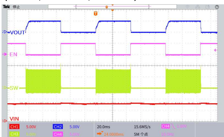
Figure 25. Start or Shutdown Using EN Pin
