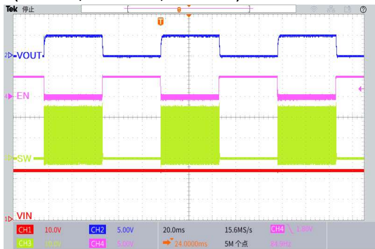
Figure 27. Start or Shutdown Using EN Pin
