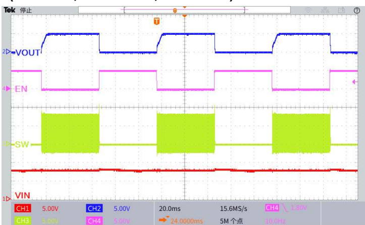
Figure 26. Start or Shutdown Using EN Pin
