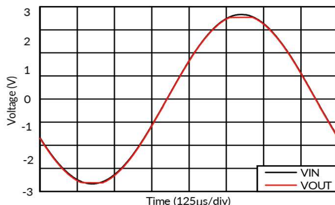
Figure 17. Output Waveform Devoid of Phase Reversal During an Input Overdrive Condition
